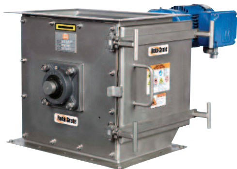
A Rota-Grate separator continuously rotates magnetic tubes through the material to eliminate bridging.
